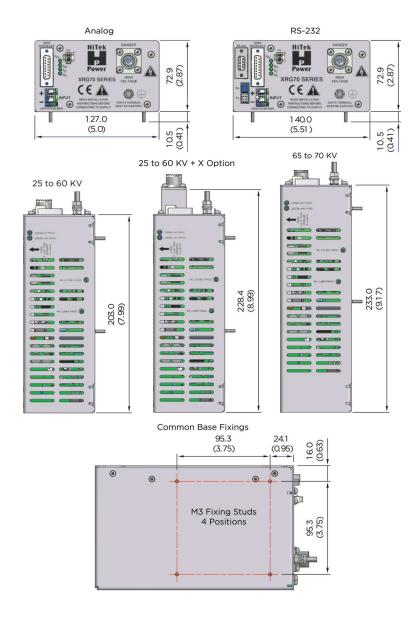
Drawing dimensions are in mm (inches). HV output cable available upon request.
