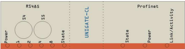
Picture 2: Front panel: Rotary switches and LEDs
