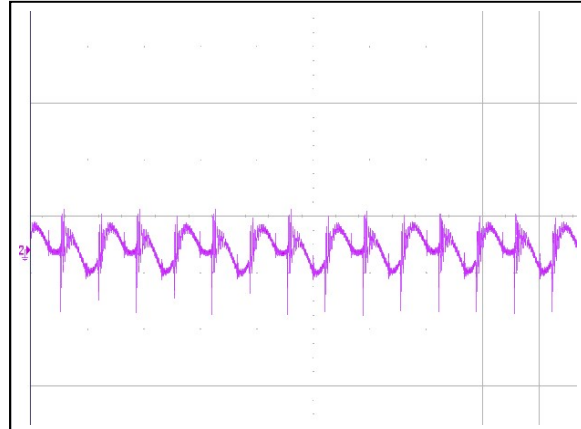
Figure 2: AGF600-48S28-6L Ripple and Noise Measurement Ch 2: Vo (50ns/div, 50mV/div)
