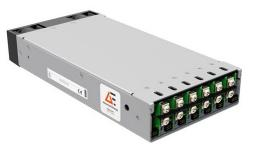
CoolX, in particular its low profile 1U height greatly eased the customer integration of the power supply in the system. With its exceptional low line power output of 1350 W, the CoolX was approximately 40% smaller than the competitor offerings. Weighing just 1.5 kg, it helped reduce the overall system weight of the tower and console. The customer opted for the low leakage current version (<150 uA), which ensured their system leakage current was well below the 300 uA safety limit.
