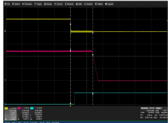
Figure 8: LCM3000L-T Turn Off Characteristic via INH_EN Vin = 264Vac Load: Io = 125A (12V), Isb = 2A Ch 1: INH_EN Ch 2: Vo Ch 3: G_DCOK_C
