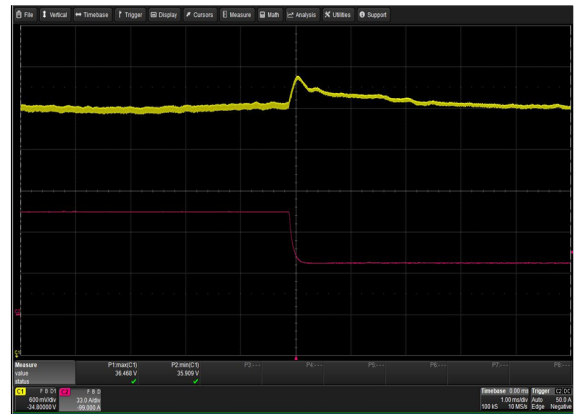
Figure 52: LCM3000U-T Transient Response - Vo Deviation 100% to 50% load change 1A/uS slew rate Vin = 230Vac Ch 1: Vo Ch 2: Io
