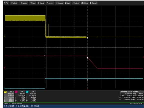
Figure 78: LCM30007-T Turn Off Characteristic via INH_EN Vin = 264Vac Load: Io = 41.7A (72V), Isb = 2A Ch 1: INH_EN Ch 2: Vo Ch 3: G_DCOK_C
