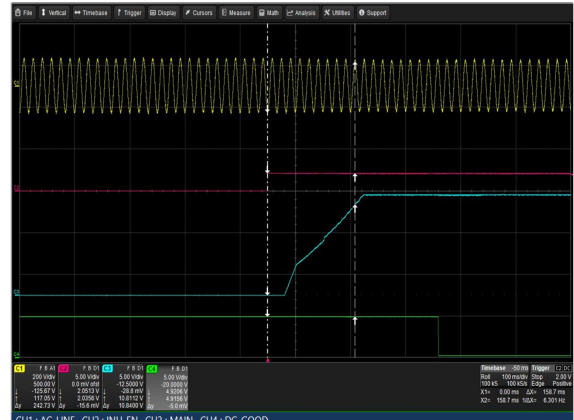
Figure 2: LCM3000L-T Turn-on delay via INH_EN Vin = 90Vac Load: Io = 125A (12V), Isb = 2A Ch 1: Vin Ch 2: INH_EN Ch 3: Vo Ch 4: G_DCOK_C
