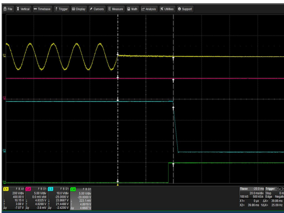
Figure 33: LCM3000Q-T Hold-up Time Vin = 90Vac Load: Io = 62.5A (24V), Isb = 2A Ch 1: Vin Ch 2: Vsb Ch 3: Vo Ch 4: G_DCOK_C
