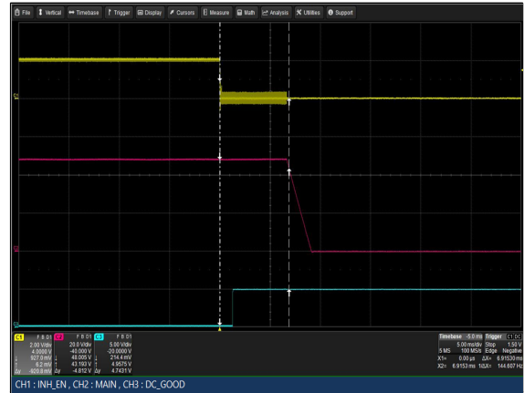
Figure 64: LCM3000W-T Turn Off Characteristic via INH_EN Vin = 264Vac Load: Io = 62.5A (48V), Isb = 2A Ch 1: INH_EN Ch 2: Vo Ch 3: G_DCOK_C
