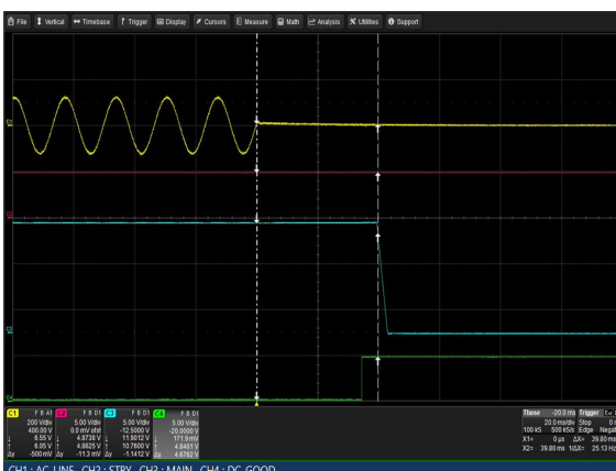
Figure 5: LCM3000L-T Hold-up Time Vin = 90Vac Load: Io = 125A (12V), Isb = 2A Ch 1: Vin Ch 2: Vsb Ch 3: Vo Ch 4: G_DCOK_C
