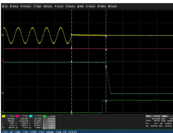
Figure 47: LCM3000U-T Hold-up Time Vin = 90Vac Load: Io = 41.7A (36V), Isb = 2A Ch 1: Vin Ch 2: Vsb Ch 3: Vo Ch 4: G_DCOK_C
