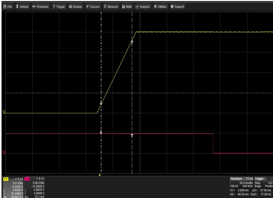
Figure 49: LCM3000U-T Output Voltage Startup Vin = 264Vac Load: Io = 83.3A (36V), Isb = 2A Ch 1: Vo Ch 2: G_DCOK_C
