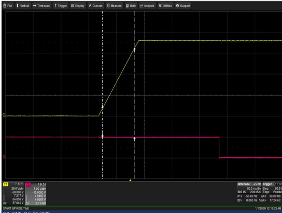
Figure 77: LCM30007-T Output Voltage Startup Vin = 264Vac Load: Io = 41.7A (72V), Isb = 2A Ch 1: Vo Ch 2: G_DCOK_C
