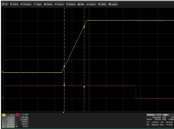
Figure 63: LCM3000W-T Output Voltage Startup Vin = 264Vac Load: Io = 62.5A (48V), Isb = 2A Ch 1: Vo Ch 2: G_DCOK_C
