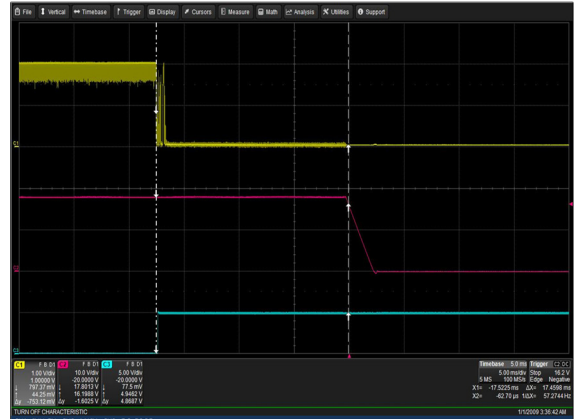
Figure 22: LCM30008-T Turn Off Characteristic via INH_EN Vin = 264Vac Load: Io = 166.7A (18V), Isb = 2A Ch 1: INH_EN Ch 2: Vo Ch 3: G_DCOK_C
