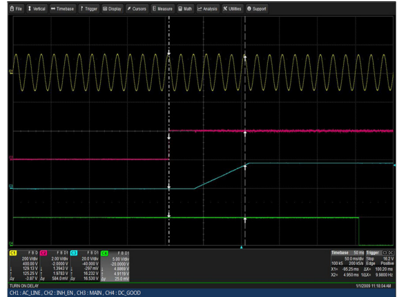
Figure 16: LCM30008-T Turn-on delay via INH_EN Vin = 90Vac Load: Io = 83.3A (18V), Isb = 2A Ch 1: Vin Ch 2: INH_EN Ch 3: Vo Ch 4: G_DCOK_C
