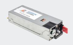
Advanced Energy's Artesyn CSU front end series is designed to provide a flexible power conversion solution for compute, storage, and networking equipment in the common redundant power supply (CRPS) form factor. This series of AC-DC products is housed in the industry standard 1U x 73.5 mm x 185 mm CRPS form factor. Featuring a 1600 W rated power, the model can cover cost-sensitive entry level systems, or power hungry applications where there are space constraints.
