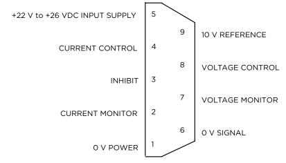
The above pinout diagram is view looking at the connector pins.
