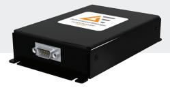
The HiTek Power<sup>®</sup> PSM10 series is a range of versatile high voltage component power supply modules equally suited to both laboratory and development work, as well as for specification in OEM equipment. Powered from 24 VDC, these units allow full range control and monitoring of voltage and current via 0 to 10 V analog signals and inhibit signal input. Positive or negative polarity models up to 15 kV are available with customer-defined derivatives upon request.
