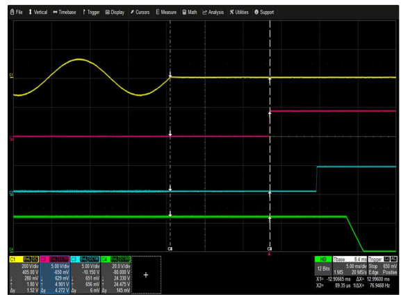
Figure 39: μMP16C-SKQ-SKQ-30-A AC OK Delay - Turn off Vin = 90Vac Load: Io = 41.66A I SB = 0A Turn On Phase = 90° Ch 1: V IN Ch 2: Input AC OK Ch 3: Global DC OK Ch 4: Vo
