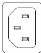
IEC Connector C14 (C)
