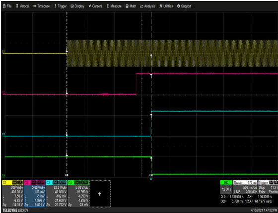
Figure 30: μMP16C-SKQ-SKQ-30-A Turn-on delay via AC mains V_{in} = 90V_{ac} Load: I_o = 41.66A I_{SB} = 2A Ch 1: AC Mains Ch 2: V_{SB} Ch 3: V_O Ch 4: Global DCOK
