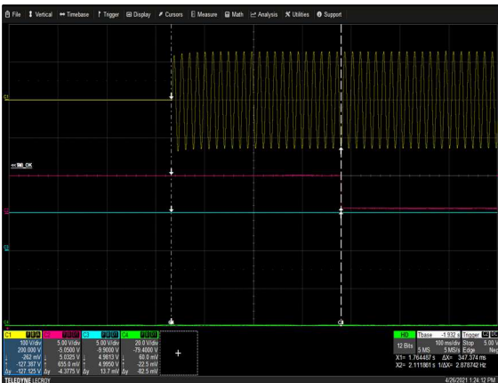
Figure 27: μMP10T-S2Q-S2Q-S2Q-S2Q-S2Q-90-A AC OK Delay - Turn on V_{in} = 90Vac Load: I_o = 41.66A Ch 1: V_{IN} Ch2: Input AC OK Ch3: Global DC OK Ch4: V_o
