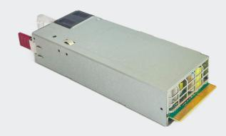
Advanced Energy's Artesyn CSU front end series is designed to provide a flexible power conversion solution for compute, storage, and networking equipment in the modular hardware common redundant power supply (M-CRPS). The 2400 W model is in the standard 1 U x 73.5 mm x 185 mm form factor. The series of power supply can cover cost-sensitive entry level systems, or power hungry applications where there are space constraints.
