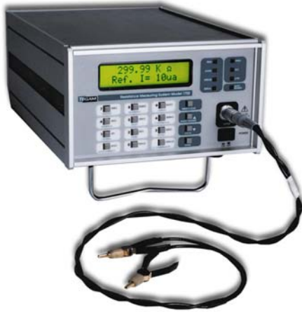
Figure 3 - The TEGAM Model 1750 is the fastest digital milliohmmeter in the industry. Capable of measuring from 100 nΩ to 20 MΩ the 1750 is optimized for automated testing of resistors, fuses, welds, wire bonds, mechanical bonds and other resistive elements. A comparator, control I/Os, RS232, RS422, and GPIB interface are included for compatibility with many common PLC or industrial control types.
