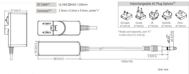
Note: The DC cable is 18AWG for 9 V and 12 V models.
