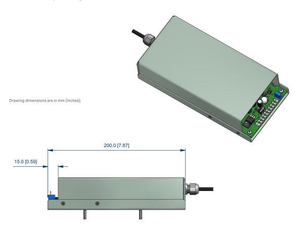
MOUNTING: 2 OFF M4 STUDS; LENGTH AND POSITION AS SHOWN DIMENSIONS  $\operatorname{mm}\left(\operatorname{in}\right)$
