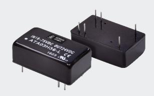
Advanced Energy's Artesyn ATA series 10 watt isolated DC-DC converters are suitable for a diverse range of low power applications, including data communication, telecommunication and computer peripheral equipment, industrial automation and mobile battery-powered systems. The series comprises 14 variants, each of which is available in a mini dual-in-line package for through-hole mounting.
