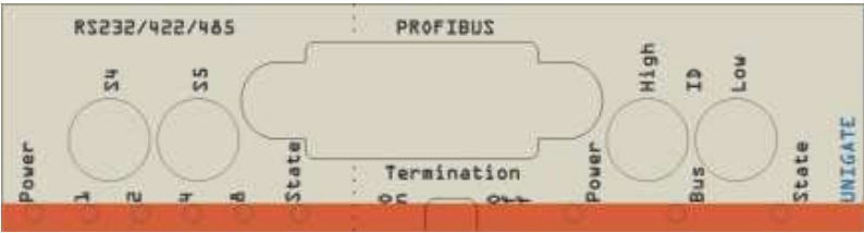
Picture 2: Front panel: Rotary switches and LEDs
