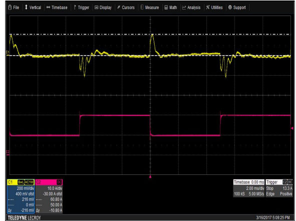
Figure 19: LCM300N Transient Response - Vo Deviation 100% to 50% load change 1A/uS slew rate Vin = 230Vac Ch 1: Vo Ch 2: Io
