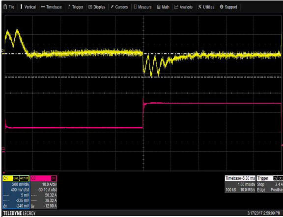
Figure 7: LCM300L Transient Response - V_O Deviation 50% to 100% load change 1A/uS slew rate V_{in} = 230V_{ac} Ch 1: V_O Ch 2: I_O
