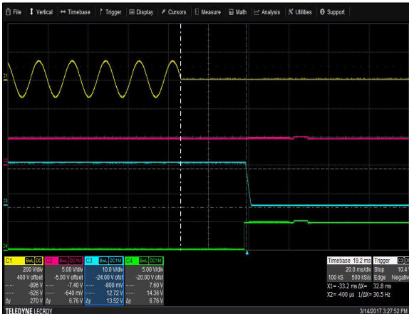
Figure 14: LCM300N Hold-up Time Vin = 90Vac / 47Hz / 0° Load: IO = 20A (15V), ISB = 2A (5V) Ch 1: AC Mains Ch 2: VSB Ch 3: VO Ch 4: G_DCOK_C
