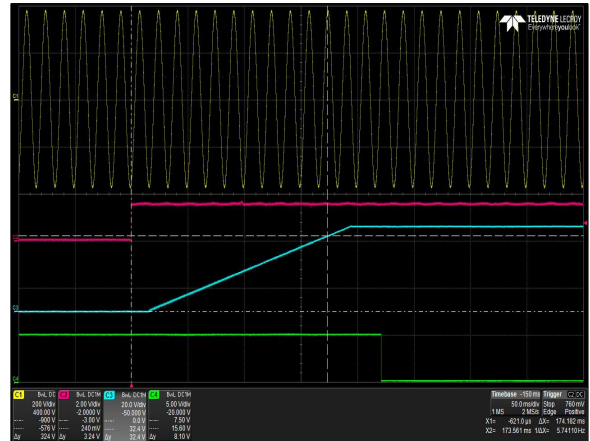
Figure 35: LCM300U Turn-on delay via INH_EN Vin = 90Vac Load: Io = 8.4A (36V), I SB = 2A (5V) Ch 1: AC Mains Ch 2: INH_EN Ch 3: Vo Ch 4: G_DCOK_C
