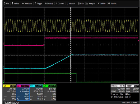
Figure 13: LCM300N Turn-on delay via INH_EN Vin = 90Vac Load: IO = 20A (15V), ISB = 2A (5V) Ch 1: AC Mains Ch 2: INH_EN Ch 3: VO Ch 4: G_DCOK_C
