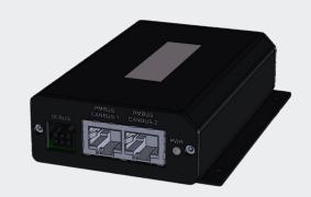
Modbus RTU communication is suitable for long distance data transmittion in electrically noisy environments. Advanced Energy's Artesyn PowerPro Dongle support Modbus RTU communication for many Artesyn power supply series, such as NeoPower, LCM10K, LCM4000HV, iTS and iHP series. It converts CANbus/CANopen and PMbus protocols to the Modbus input on the PSU\*.
