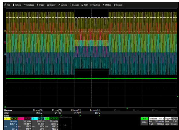
Figure 12: ORV3 Shelf Ride Through Test (5 PSUs in the shelf) Vin = 230Vac to 160V (1s) to 230Vac (L-N) Io = 300A Ch 1: Vin (L1-N) Ch 2: Vin (L2-N) Ch3: Vin (L3-N) Ch4:Vo
