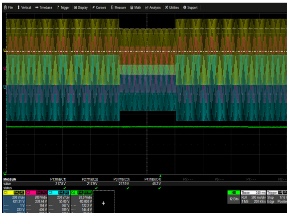
Figure 11: ORV3 Shelf Ride Through Test (6 PSUs in the shelf) Vin = 230Vac to 160V (1s) to 230Vac (L-N) Io = 300A Ch 1: Vin (L1-N) Ch 2: Vin (L2-N) Ch3: Vin (L3-N) Ch4:Vo
