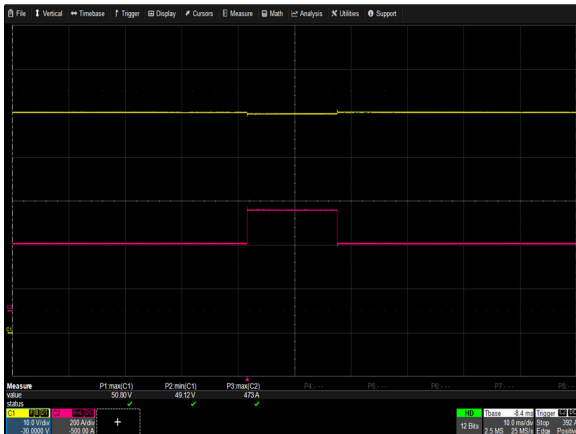
Figure 15: ORV3 Shelf Pulse Load (6 PSUs in the shelf) Vin = 400Vac(L-L) Io = 300A to 450A (16ms) single pulse Ch 1:Vo Ch 2: Io (slew rate: 5A/us)
