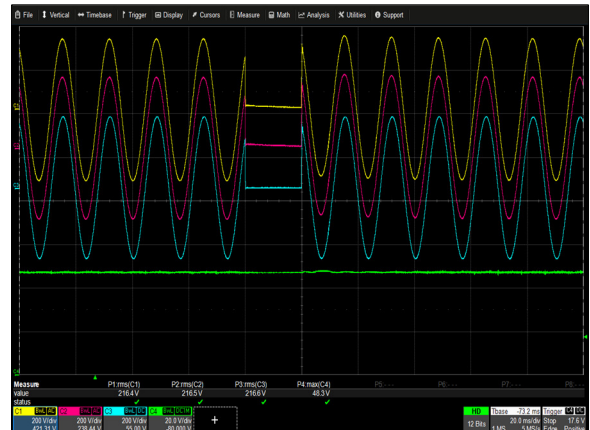
Figure 8: ORV3 Shelf Ride Through Test (5 PSUs in the shelf) Vin = 230Vac to 0V (20ms) to 230Vac (L-N) Io = 300A Ch 1: Vin (L1-N) Ch 2: Vin (L2-N) Ch3: Vin (L3-N) Ch4:Vo
