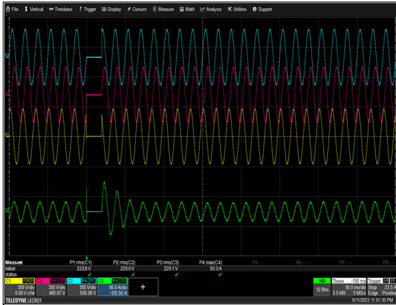
Figure 19: ORV3 Shelf Inrush Current Vin = 230Vac(L-N) (3 phases drop for 20ms) Io = 150A Ch 1: Vin (L1-N) Ch 2: Vin (L2-N) Ch3: Vin (L3-N) Ch4:in
