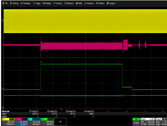
Figure 21: ORV3 Shelf Over Power/Current Protection Vin = 400Vac(L-L) Io = 432A(100ms) to 396A(9.9s) to 40A(1.14s) Ch 1:Vin Ch 2: in Ch3:Vo Ch4:Io
