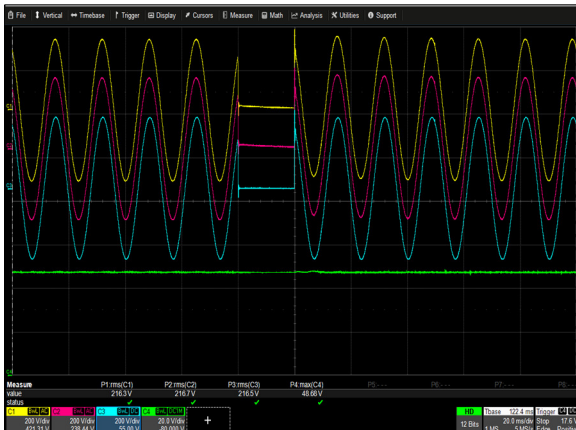
Figure 7: ORV3 Shelf Ride Through Test (6 PSUs in the shelf) Vin = 230Vac to 0V (20ms) to 230Vac (L-N) Io = 300A Ch 1: Vin (L1-N) Ch 2: Vin (L2-N) Ch3: Vin (L3-N) Ch4:Vo
