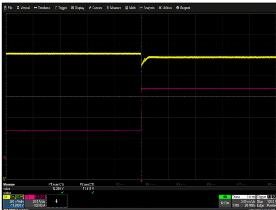
Figure 11: CSU2000AT-3-100 Transient Response - V_O Deviation 65.56A to 163.9A (40% to 100%) 1A/\mu s slew rate Vin = 230Vac Ch 1: V_O Ch 2: I_o
