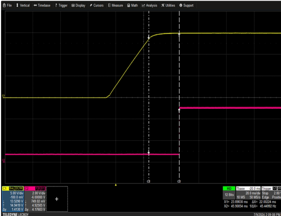
Figure 33: NP08W1-1MN0-00-A-0 Output Voltage Startup Characteristic Load: I_o = 26.6A Ch 1: V_o Ch 2: ISO_POWER_GOOD
