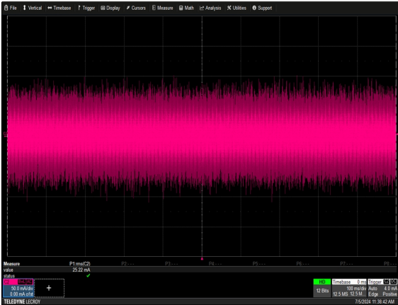
Figure 58: NP08W1-1MW0-00-A-0 Ripple and Noise Measurement Load: R = 5.78 ohm Ch 2: I O
