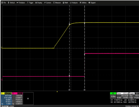
Figure 51: NP08W1-1MW0-00-A-0 Output Voltage Startup Characteristic Load: I_o = 8.3A Ch 1: V_o Ch 2: ISO_POWER_GOOD
