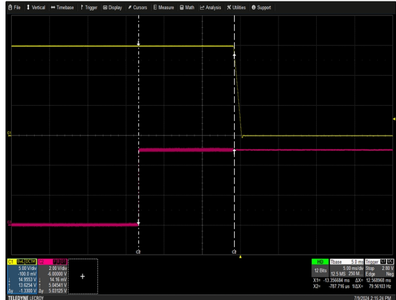
Figure 34: NP08W1-1MN0-00-A-0 Turn Off via Module Inhibit Load: I_o = 26.6A Ch 1: V_o Ch 2: Module Inhibit
