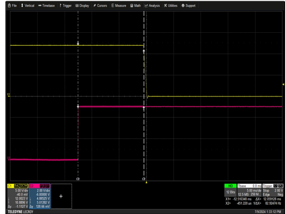
Figure 25: NP08W1-1ML0-00-A-0 Turn Off via Module Inhibit Load: I_o = 33.3A Ch 1: V_o Ch 2: Module Inhibit
