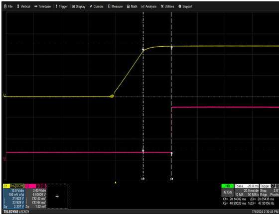
Figure 42: NP08W1-1MQ0-00-A-0 Output Voltage Startup Characteristic Load: I_o = 16.6A Ch 1: V_o Ch 2: ISO_POWER_GOOD
