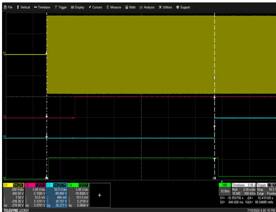
Figure 3: NP08W1-1MW0(8)-00-18P-A-0 Turn-on delay via AC mains Vin = 264Vac Load: I_o = 66.67A I_{SB} = 1A Ch 1: AC Mains Ch 2: V_{SB} Ch 3: V_o Ch 4: G_PG00D
