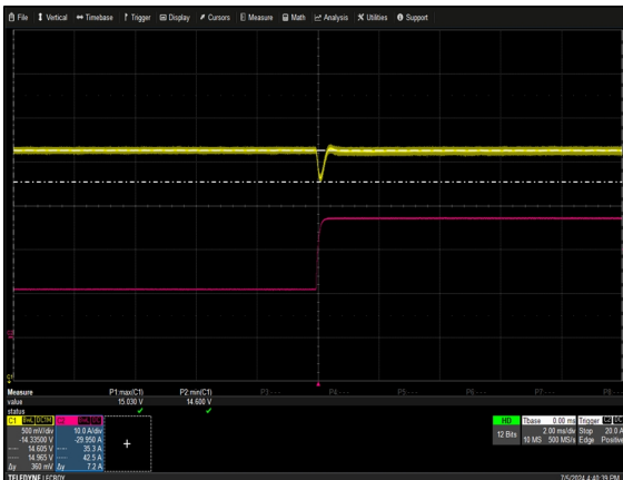
Figure 35: NP08W1-1MN0-00-A-0 Transient Response - V_o Deviation 40% to 100% load change, 1A/ \mu s slew rate Ch 1: V_o Ch 2: I_o
