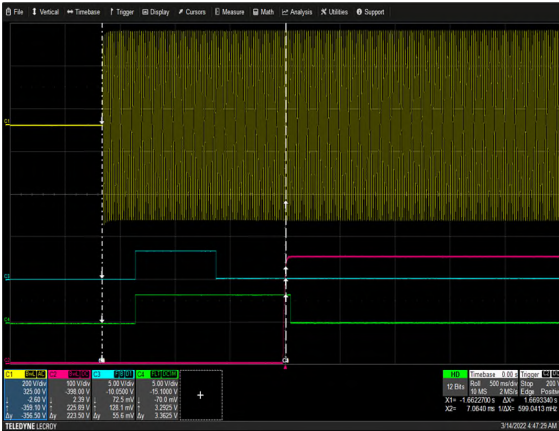
Figure 1: LCM4000HV-T Turn-on delay via AC mains Vin = 311Vac Load: Io = 16A Ch 1: Vin Ch 2: Vo Ch 3: AC_OK Ch 4: DC_OK
