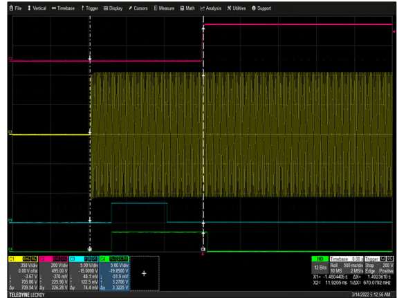
Figure 2: LCM4000HV-T Turn-on delay via AC mains Vin = 520Vac Load: Io = 16A Ch 1: Vin Ch 2: Vo Ch 3: AC_OK Ch 4: DC_OK
