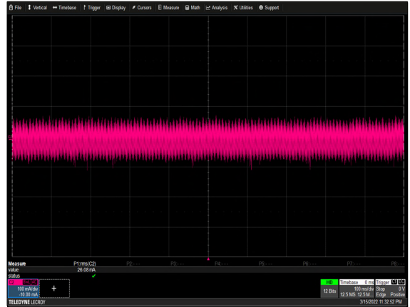
Figure 11: LCM4000HV-T Ripple and Noise Measurement Vin = 380Vac Load: R = 15.62 ohm Ch 2: io
