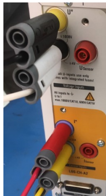
Figure 5: CA-70-5 and CA-71-5 connections to Power Analyzer
