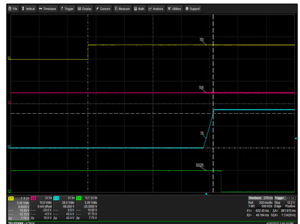
Figure 16: LCC1200-48U-9P Turn-on delay via INH_EN Vin = 264Vac Load: Io = 25A (48V), I SB = 1.5A (5V) Ch 1: INH_EN Ch 2: V SB Ch 3: V 0 CH 4: G_DCOK_C
