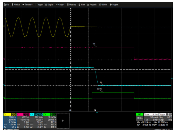
Figure 6: LCC1200-28U-9P Hold-up Time Vin = 264Vac Load: Io = 42.9A (28V), I SB = 1.5A (5V) Ch 1: AC Mains Ch 2: V SB Ch 3: V O CH 4: G_DCOK_C
