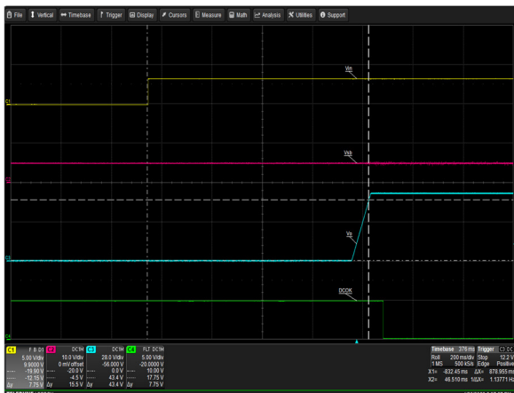
Figure 15: LCC1200-48U-9P Turn-on delay via INH_EN Vin = 90Vac Load: Io = 16.67A (48V), I SB = 1.5A (5V) Ch 1: INH_EN Ch 2: V SB Ch 3: V 0 CH 4: G_DCOK_C
