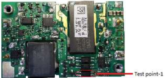
Figure 12 Temperature test points
