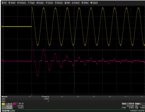
Figure 7: CSU1600AT-3-100 Inrush Current V_{in} = 240V_{ac} Load: I_o = 0A , Turn on at 90 deg Ch 1: V_{IN} Ch 2: I_{IN}
