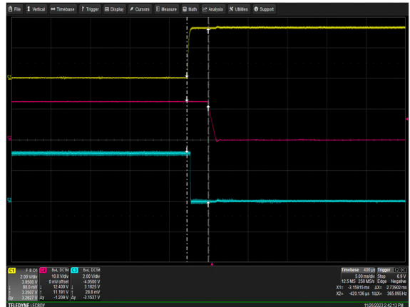
Figure 10: CSU1600AT-3-100 Turn Off Characteristic via PS_ON Load: I_o = 131.1A I_{SB} = 3.5A Ch 1: PS_ON Ch 2: V_o Ch 3: PW_OK
