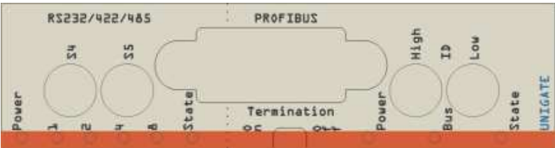
Picture 2: Front panel: Rotary switches and LEDs
