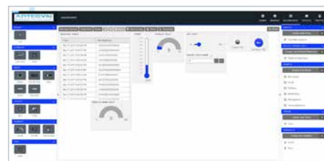
Typical Dashboard. User configurable with drag and drop widgets assignable to any device, script timer or variable.
