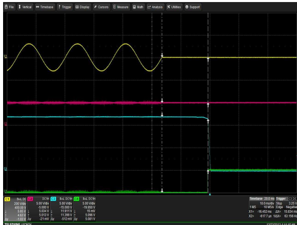
Figure 3: LCM1500L-T-4 Hold-up Time Vin = 90Vac / 47Hz / 0° Load: lo = 125A (12V), Isb = 2A (5V) Ch 1: Vin Ch 2: Vsb Ch 3: Vo Ch 4: G_DCOK_C
