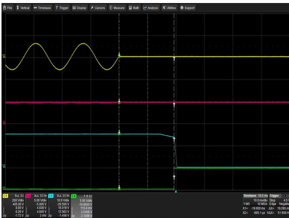
Figure 14: LCM1500N-T-4 Hold-up Time Vin = 90Vac / 47Hz / 0° Load: lo = 100A (15V), Isb = 2A (5V) Ch 1: Vin Ch 2: Vsb Ch 3: Vo Ch 4: G_DCOK_C
