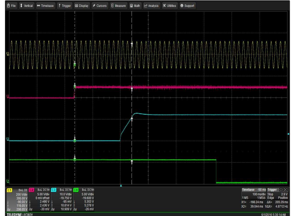
Figure 2: LCM1500L-T-4 Turn-on delay via INH_EN Vin = 90Vac Load: lo = 125A (12V), Isb = 2A (5V) Ch 1: Vin Ch 2: INH_EN Ch 3: Vo Ch 4: G_DCOK_C
