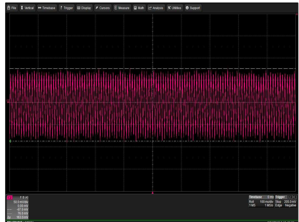
Figure 43: LCM1500R-T-4 Ripple and Noise Measurement Vin = 115Vac Load: I_o = 53.6A (28V), I_{SB} = 2A (5V) Ch 2: Vo
