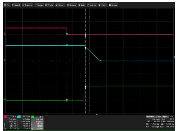
Figure 6: LCM1500L-T-4 Turn Off Characteristic via INH_EN Load: lo = 125A (12V), Isb = 2A (5V) Ch 2: INH_EN Ch 3: Vo Ch 4: G_DCOK_C
