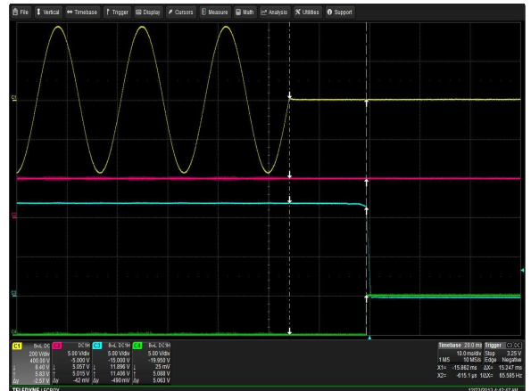
Figure 4: LCM1500L-T-4 Hold-up Time Vin = 264Vac / 60Hz / 0° Load: lo = 125A (12V), Isb = 2A (5V) Ch 1: Vin Ch 2: Vsb Ch 3: Vo Ch 4: G_DCOK_C
