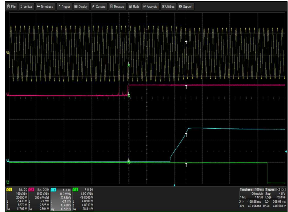
Figure 13: LCM1500N-T-4 Turn-on delay via INH_EN Vin = 90Vac Load: lo = 100A (15V), Isb = 2A (5V) Ch 1: Vin Ch 2: INH_EN Ch 3: Vo Ch 4: G_DCOK_C
